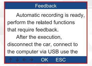
Next: Press EXIT Button and return to the main menu. Choose [OBDII] menu to detecting again and it will record the data.
